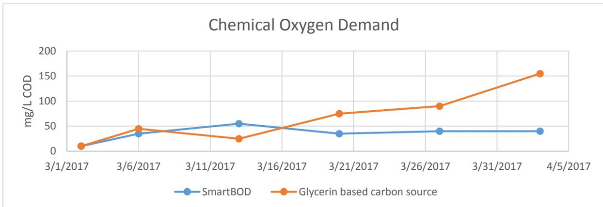
FIGURE 5: CHEMICAL OXYGEN DEMAND IN REACTOR EFFLUENT
