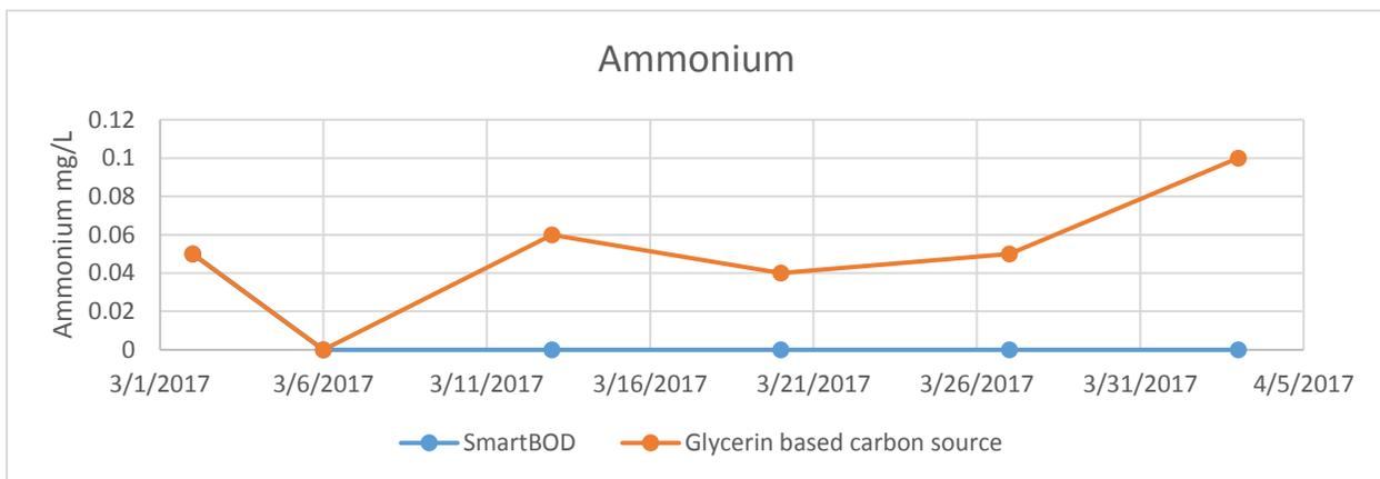
FIGURE 3: AMMONIUM CONCENTRATION IN REACTOR EFFLUENT
