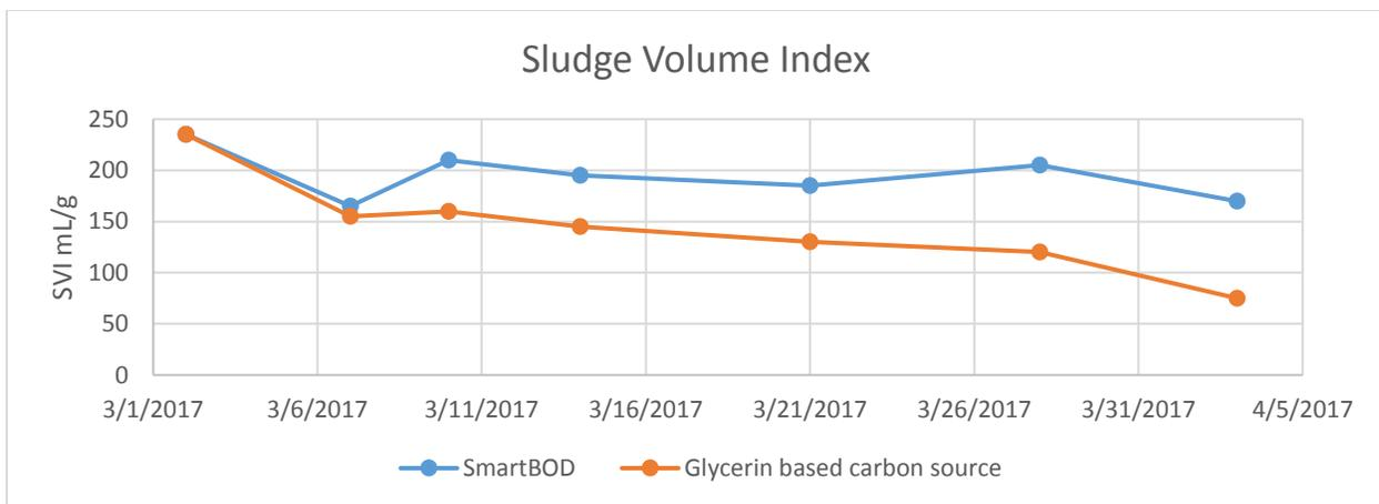
**FIGURE 6: MIXED LIQUOR SLUDGE VOLUME INDEX**
